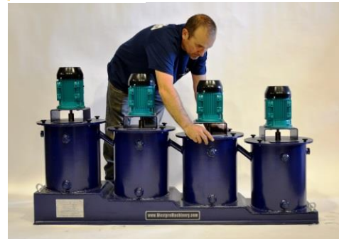
PILOT STAGE LEACH TANKS
