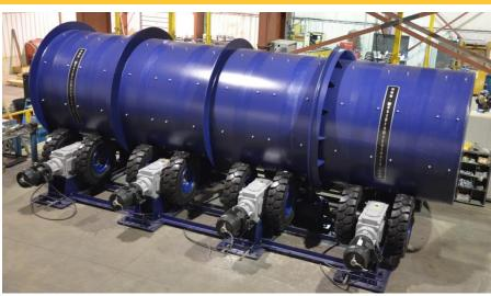
Tire drive agglomerators eliminate the use of riding rings and use rubber tires. Tire drive agglomerators are engineered to ensure quality agglomeration of standard materials. Finite process control is available with the VFD package.
