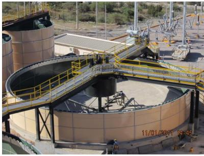
Westpro's thickeners are equipped with new generation hydraulic drives, high capacity feedwells, and low drag-high capacity rakes to deliver superior solids settling performance. Along with their robust construction, Westpro's thickeners ensure superior performance in high-torque applications.
