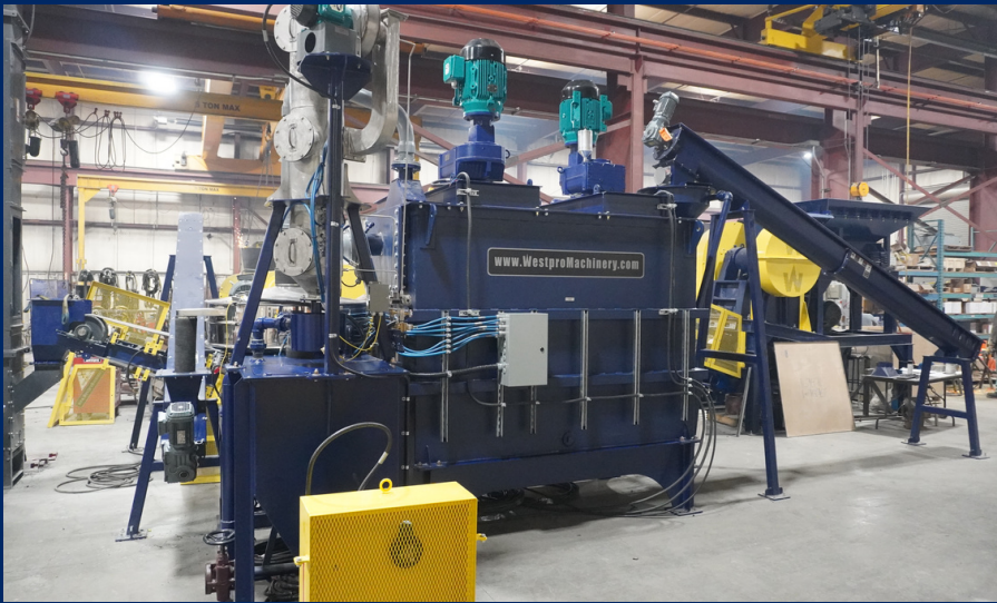
SLAKER DT-48 with a capacity up to 6500 KG/HR
