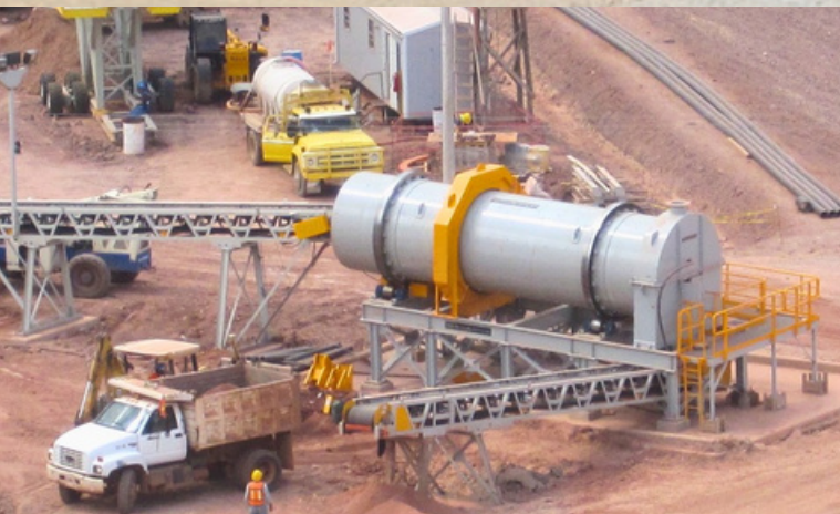
Top: Two (2) 3m (10ft) diameter chain drive Agglomerators at a gold heap operation in Mexico Bottom Left: 2.4m (8ft) diameter chain drive Agglomerator at a gold heap leach operation in Mexico Bottom Right: 2.4m (8ft) diameter tire drive Agglomerator at a copper heap leach operation in Mexico
