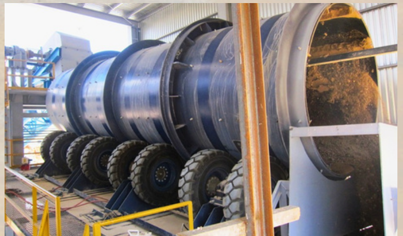
Top: Two (2) 3m (10ft) diameter chain drive Agglomerators at a gold heap operation in Mexico Bottom Left: 2.4m (8ft) diameter chain drive Agglomerator at a gold heap leach operation in Mexico Bottom Right: 2.4m (8ft) diameter tire drive Agglomerator at a copper heap leach operation in Mexico
